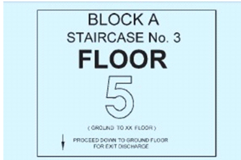
14a. Example of a Stairway Marking Sign (Floor Indication Board)
